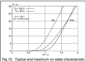
Fig. 10. Typical and maximum on-state characteristic.
