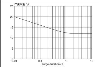
Fig.5. Maximum permissible repetitive rms on-state current  $I_{T(RMS)}$ , versus surge duration, for sinusoidal currents, f = 50 Hz;  $T_{mb} \le 103 ^{\circ}\text{C}$ .
